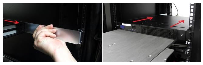
**CAUTION!** Support the weight of the appliance with the hydraulic lift until all four brackets are secured.
