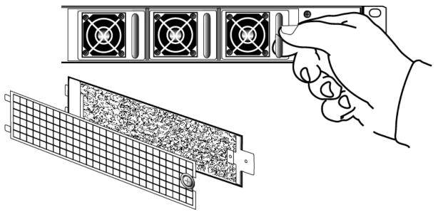
5. After slight initial resistance, the fan module should easily slide free of the appliance.
