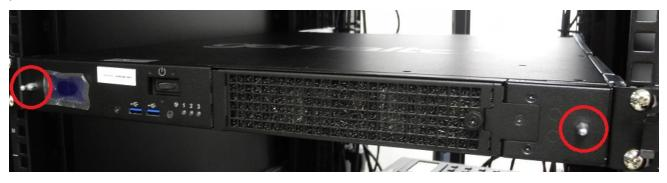
2. Turn the keys to the vertical position to lock the bezel.
