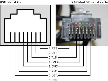
**NOTE** The Luna Network HSM 7 appliance does not implement serial handshaking, so RTS/CTS (pins 1 and 8) and DSR/DTR (pins 7 and 2) are not used for a successful connection. The important signals are TxD and RxD (pins 3 and 6).
