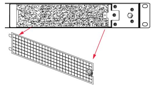
2. With the air filter exposed, it is easy to grasp the mesh with fingers and tug it free. The mesh is flexible and is held in its cavity only by friction. If it is dusty, handle carefully so as not to dislodge any dirt that could then be sucked in by the fans.
