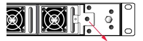
2. The fan retainer is anchored at its left by two tabs - swing the retainer out like a door, and remove it. There is no need to separate the filter mesh and its retainer from the larger fan retainer; the assembly can come out as one piece. The illustration below happens to show them separated.
