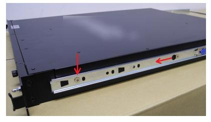
6. Fit the sliding rails onto the rack mounts until they lock into place.
