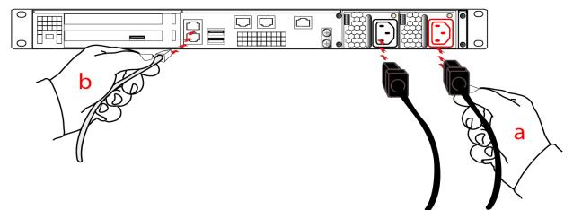
2. If you have a multifactor quorum-authenticated Luna Network HSM 7, connect the Luna PED directly to the HSM card's USB port (on the rear panel's left side), using the included USB-to-MiniUSB PED cable. See also Local PED Setup. If you have a password-authenticated HSM, skip to the next step.
