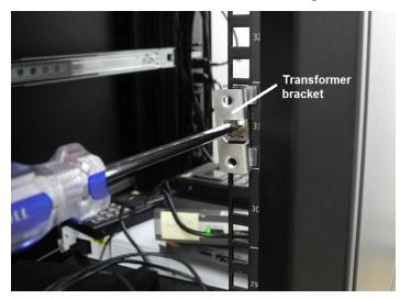
5. Loosely thread two small flat-headed screws into each side of the Luna Network HSM 7. Fit each sliding rail over the screw heads and slide it forward into place before tightening the screws. Fasten each sliding rail with a third screw where it lines up with the hole in the HSM chassis.
