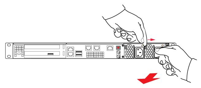
Withdraw the power supply completely, using your other hand to support the body of the power supply as it emerges.
