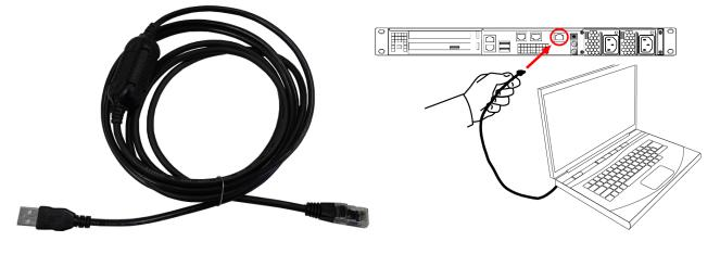
NOTE Do not connect the serial cable to one of the Ethernet ports.
