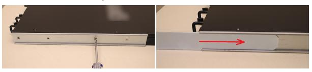
4. Install the two sliding rear brackets in your equipment rack using four rack mounting screws.
